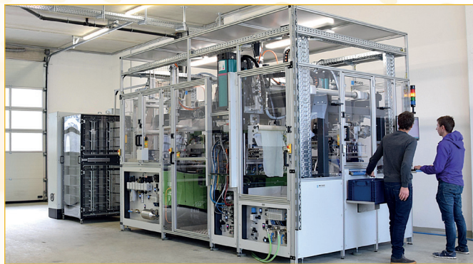
Fibionic's automated system is able to position load path aligned fibres in milliseconds. In short: higher performance, lower cost and almost zero waste
